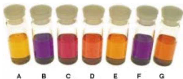
Figure 1. Photograph showing the color of dilute solutions of 1,2-diaminoanthraquinone in dichloromethane ( [\text{quinone}] = 1.0 \times 10^{-4} \text{ M} ). A) Before addition of the anion. After addition of 100 equivalents of B) fluoride, C) chloride, D) bromide, E) iodide, F) phosphate, and G) sulfate ions. All anions were added in the form of their tetrabutylammonium salts.
